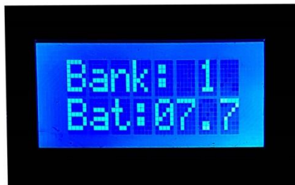
2. The bank of control plate and the state of battery
